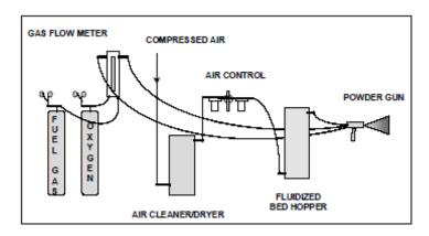
Figure 2-4. Typical combustion powder gun installation
