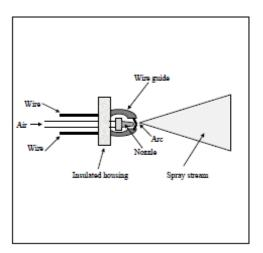
Figure 2-7. Typical two-wire arc spray gun
