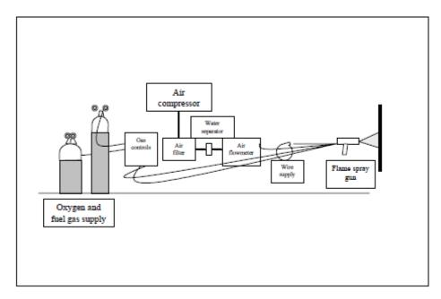
Figure 2-2. Typical flame spray system
