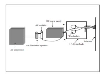
Figure 2-6. Typical two-wire arc spray system
